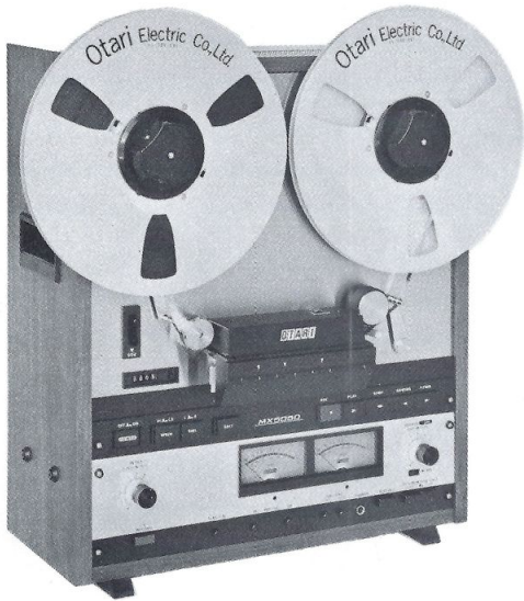
MX-5050-FL. Single channel version of the MX-5050 with full-track record and reproduce, plus an extra two track reproduce head and reproduce electronics channel for playing back two channel tapes.
