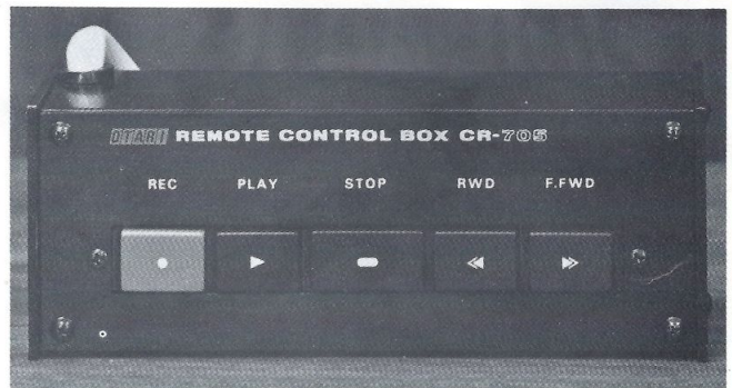
Remote control unit for all transport functions except speed change.
