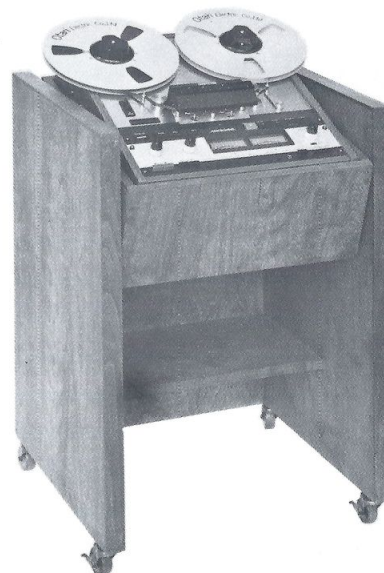
Floor cabinet with casters converts the MX-5050 into a studio console machine.
